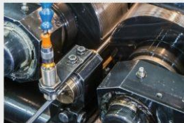
Core competence thread rolling: run-through process.
