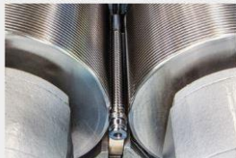
Core competence thread rolling: infeed process.
